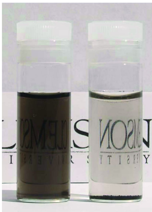
Figure 1. Visual comparison on the aqueous dispersions of Gal 2 MWNT (left) and Gal-MWNT (right). (Adapted from ref. (34).)
